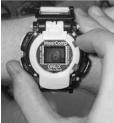
Figure 2.3 The wristwatch videoconferencing computer running the videoconferencing application underneath a transparent clock, running XF86 under the GNUX (GNU + Linux) operating system: (a) Worn while in use; (b) Close-up of screen with GNUX “cal” program running together with video window and transparent clock.
