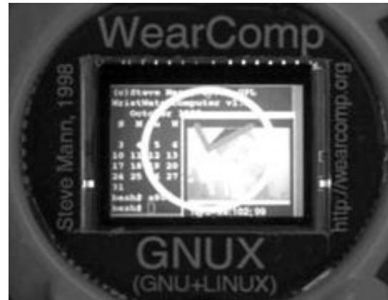
Figure 2.3 The wristwatch videoconferencing computer running the videoconferencing application underneath a transparent clock, running XF86 under the GNUX (GNU + Linux) operating system: (a) Worn while in use; (b) Close-up of screen with GNUX “cal” program running together with video window and transparent clock.
